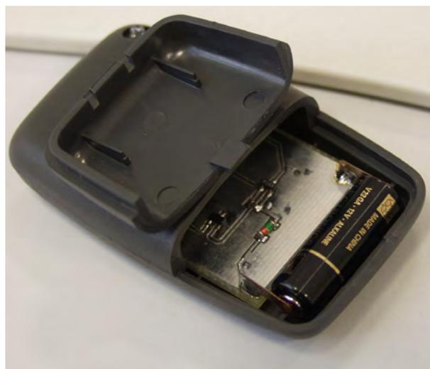
Pic. 3: Polarity of the battery
